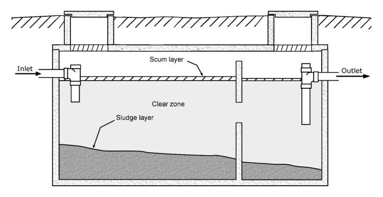
Drawing modified from CIDWT. 2009. *Installation of Wastewater Treatment Systems*. Consortium of Institutes for Decentralized Wastewater Treatment (CIDWT). Iowa State University, Midwest Plan Service. Ames, IA.
