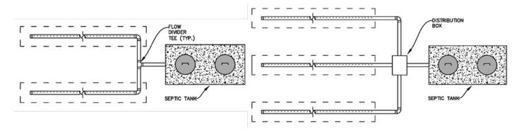
DEQ does not require installation of leachfield trenches in a straight line. In fact, it is always preferable to follow the contour of the land. Additionally, never install the leachfield in floodways, at the base of slopes, or in depressions where runoff water could flood the leachfield. Construct leachfields in areas with good surface drainage, where the water cannot pond over the leachfield.
