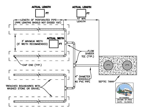
Draw your perforate pipe trench layout below or attach a separate sheet.
