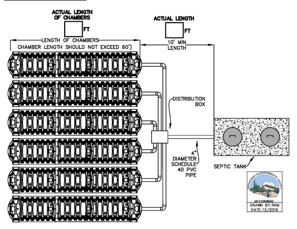
Draw your chambered bed layout below or attach a separate sheet.
